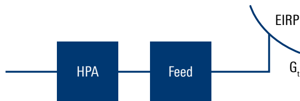
Fig. 66: SATCOM transmitter frontend
